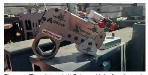
Figure 4: The alkitronic X Driver with its flat design is ideal for working in tight spaces.
