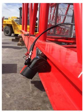
Figure 3: Test with the hydraulic torque multiplier AT from alkitronic.
