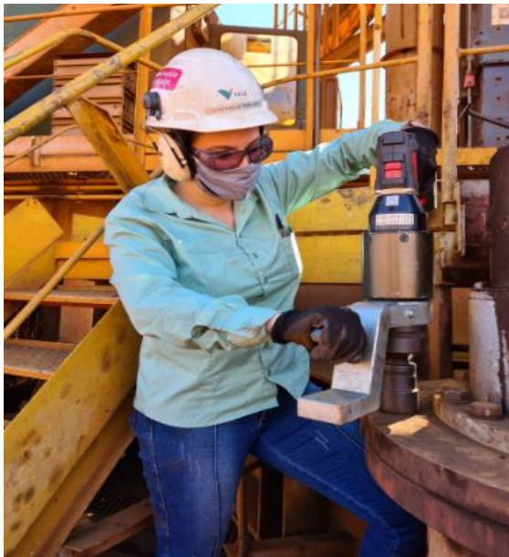
Figure 2: A worker maintains a machine with an alkitronic® torque multiplier EAF.
